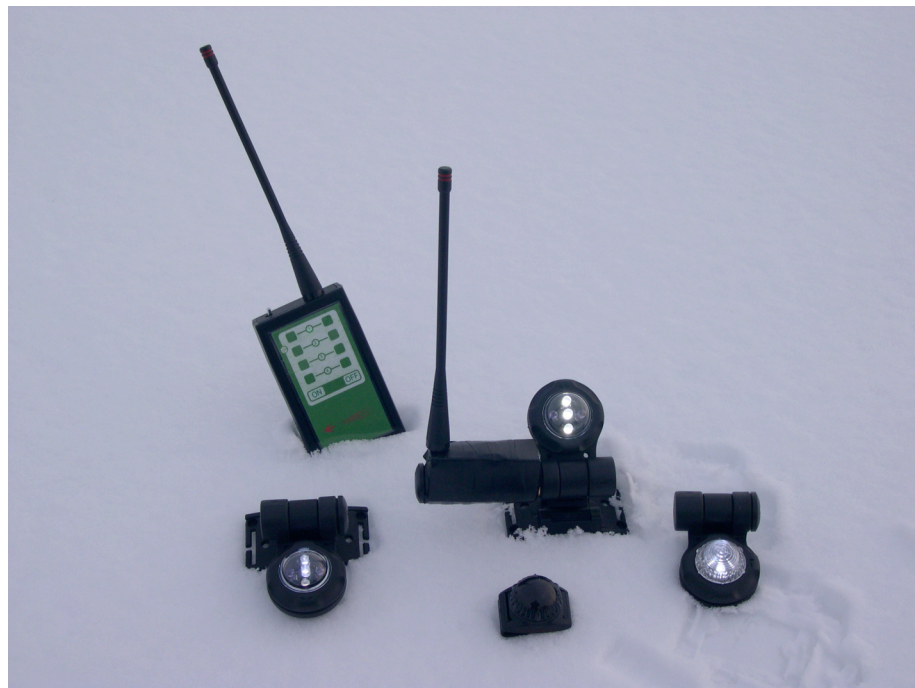
Figure 2- Automated lights used for car tracking (middle bottom) and landing zone tasks
